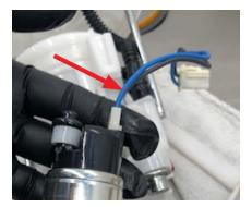
For this recall, the 2-wire (Blue / Black) fuel pump wiring harness indicated as 1-time use in the Service Manual is reused but, should be inspected for damage or any evidence of overheating (discoloration of connectors, etc.). **IMPORTANT**: If any damage e.g. distorted or melting plastic connectors, overheated wiring or terminals is identified, the harness MUST be replaced. It easily unplugs from the fuel pump.
