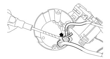
• Using 2 small flat-blade screwdrivers, **CAREFULLY** release the 2 claws securing the fuel pump to the regulator.
