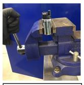
**IMPORTANT:** Remove the o-ring and spacer from the original fuel pump. The spacer is reused. Put the removed pump in a vise and crush it as shown above to eliminate any chance of it being reused.
