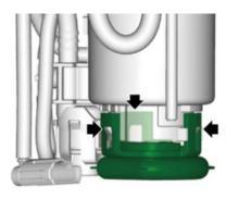
Remove the fuel pump holder then disengage the 3 claws securing the fuel pump to the filter assembly.
