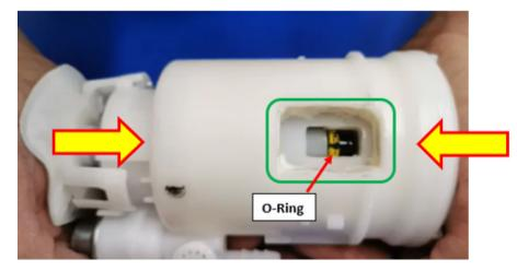
**CRITICAL TIP:** Align and press the new fuel pump **FIRMLY**, **SQUARELY** and **STRAIGHT** into the filter housing in ONE smooth, continuous motion.
