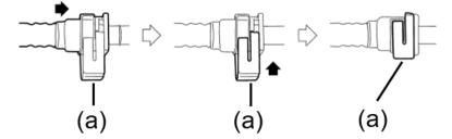
**IMPORTANT REMINDERS:** Discard the removed temporary fuel line plug as it is a one-time use item. Reusing the plug may damage the connector's internal o-ring and cause a fuel leak.
