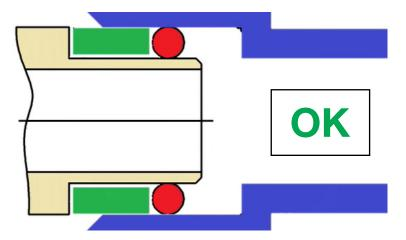
The new fuel pump is being pressed firmly and squarely into the filter housing bore and successfully "clicks" into place.
