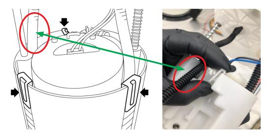
• **CAREFULLY** remove the fuel tube assembly from the fuel chamber using a small flat-blade screwdriver wrapped with protective tape as shown.
