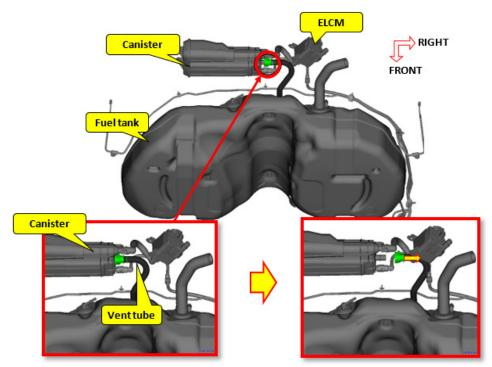
(STEP :1) Using the Redline Detection Smoke Pro (RDL-95-0051), apply 10kpa (1.45 PSI) at the vent tube. These pressures for this test are higher than those specified when confirming proper sealing of the fuel pump. Check to ensure the pressure is retained for 10 seconds. Is the pressure retained?
