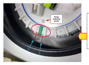
**IMPORTANT:** This photo shows the NEW ring nut and (Blue) seal plate included in the kit already in place. The ASCENT ring nut thread starting point is identified by the 3 "teeth" close together (RED circled). Align the center (Green) tooth (position mark) with the triangle  $\Delta$  mark between the molded-in hash marks on the tank (Blue arrows).
