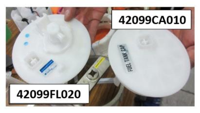
**NOTE:** When searching STIS for the applicable Service Manual procedures for reference, select **Fuel Filter REMOVAL** to get the detailed procedure for separating the pump / filter sock assembly from the complete fuel pump assembly. Fuel Filter removal is **NOT** required to complete this procedure. The replacement pumps come with a new filter sock already in place as shown here.
