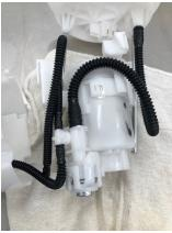
• After separating the fuel filter from the fuel chamber assembly, inspect the fuel chamber to confirm the o-ring is not still in the bore as shown here. If the o-ring remains, use a rubber -tipped or plastic (non-marring) pick tool to **CAREFULLY** remove it without scratching the fuel chamber bore.
