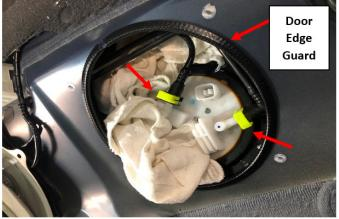
retaining clip(s) with a small flat-blade screwdriver, put a cloth over the connection and remove the line(s). Immediately install the plug(s) provided in the replacement fuel pump kits into the removed line(s) to avoid any spillage. This will help reduce the chances of post-repair customer concerns of fuel odor inside the cabin.
