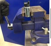
IMPORTANT: Remove the o-ring and spacer from the original fuel pump. The spacer is reused. Put the removed pump in a vise and crush it as shown here to eliminate any chance of it being reused.
