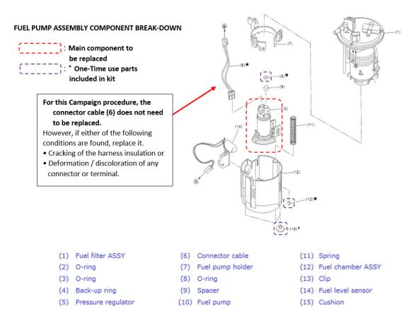
\*The 3 rubber cushions (15) on the bottom of the fuel chamber and included in the kit must be replaced as they are 1-time use.
