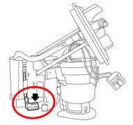
• Refit the spring **(B)** to the rod with the snap ring groove then re-install the pump / filter assembly into the fuel chamber. **IMPORTANT**: Confirm tube **(A)** is routed <u>UNDER</u> the retaining claw then lock all 3 claws in place.
