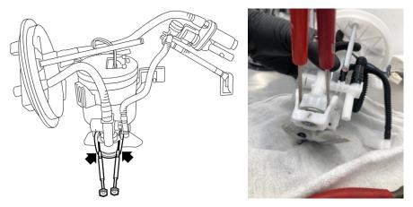
• Release the 3 remaining claws at the bottom of the fuel pump then **CAREFULLY** press down on the top of the pump to push it out the bottom of the fuel filter assembly.
