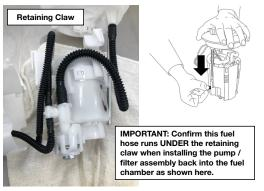
**10. CAREFULLY** refit the fuel level sensor assembly to the fuel chamber. Put the (thinner) fuel lever sensor wires into the 2 retaining clips first followed by the fuel pump wires **IN THAT ORDER.**
