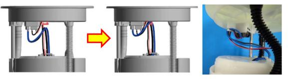
11. CRITICAL: <u>ALL</u> surfaces of the new pump assembly o-ring, top gasket, underside of the ring nut along with the surfaces described and shown below: fuel tank neck rim (A) pump flange top and bottom faces (B) and (C) must be thoroughly wiped clean and completely dried BEFORE re-installation. This will help prevent the pump from turning with the ring nut during final tightening.
