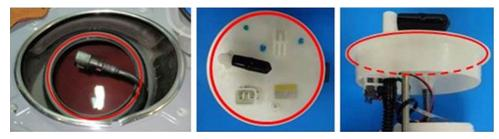
• On Impreza, start the ring nut with the indexing arrow centered between the hash marks. Tighten the ring to 96 ft. lbs. **IMPORTANT:** As the specified torque approaches, confirm the indexing arrow on the fuel pump stays between the hash marks. When successful alignment and torque are achieved, perform the height adjustment check procedure below.
