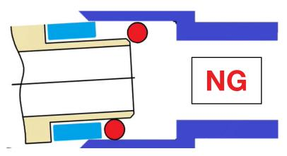
Here, the new fuel pump is being pressed into the filter housing bore at an angle which will likely result in the outlet tube butting against the shoulder of the bore the o-ring seals against followed by repeat attempts which often end up with the o-ring becoming dislodged.
