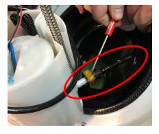
cloth. The plug is not required when replacing the complete fuel pump assembly due to the very short time the tank will be open for that repair.
