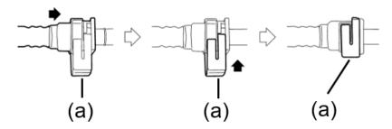
**IMPORTANT REMINDERS:** Discard the plastic fuel line plug as it is a one-time use item. Reusing the plug may damage the connector's internal o-ring and cause a fuel leak.
