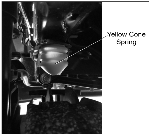
Figure 2 – Yellow Cone Spring Installation
