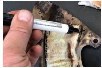
**IMPORTANT:** As each heat shield is **CAREFULLY** removed, use a permanent marker to outline the shape and positioning of each fiberglass insulation pad found on the inside of it whenever possible. A complete set of new insulation pads is included in the EPF kit and **ALL are to be replaced at reassembly**.
