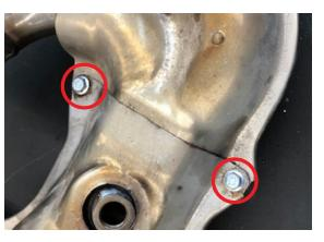
(9.6 ft. lbs.) **EXCEPT** for the two on the driver's side shield shown in the photo below. This shield covers the bellows section of the EPF and if tightened, the dimension of the bellows may be changed enough to keep the EPF assembly from fitting back onto the exhaust studs properly.
