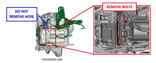
**REV. 2)** It is not necessary to remove the A/C compressor to access the cylinder #2 fuel injector harness connector. It can be disconnected with the A/C compressor installed.
