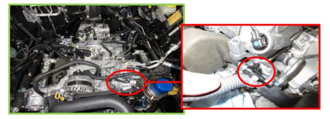
**REV. 3)** The throttle body assembly does not have to be fully removed. Remove the four mounting bolts and disconnect the wiring harness connection (**A**). The throttle body assembly can be repositioned with the pre-heater (coolant) hoses (**B**) attached to allow sufficient access. Use **CAUTION** to not damage the throttle plate during this procedure.
