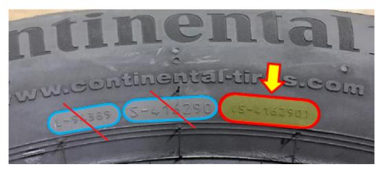
VERY IMPORTANT: When performing these inspections, <u>BOTH</u> the DOT Serial Number and the Mold Number (circled in RED, Highlighted and In Parentheses) must match those provided above. <u>If only one of the 2 numbers match</u>, the tire(s) is not affected.
