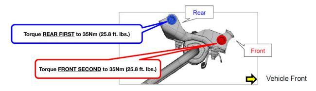
STEP 5 – Re-check the torque of the bolts in the same order as in STEP 4 (35 Nm (25.8 ft-lbs.).
