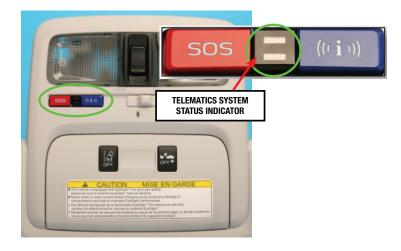
**VERY IMPORTANT:** Before attempting programming, the status of the Starlink Telematics system **MUST** be confirmed by observing the RED and GREEN indicator LEDs on the overhead console located between the Blue "i" and Red "SOS" buttons with the ignition ON.
