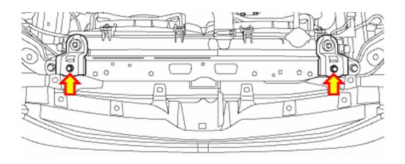
**STEP 6:** Remove the two (2) retaining bolts from the bottom of the A/C Condenser using Special Tool **73099SG000** as shown in **Step 10**.
