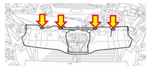
**STEP 3:** After removing the retaining clips, remove the grille bracket.
