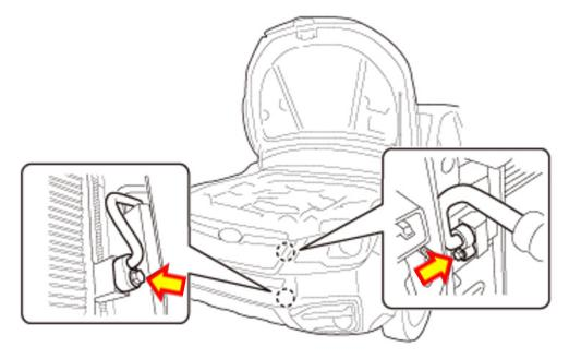
**IMPORTANT:** Using the proper size plastic plug or electrical tape, seal the ends of the removed pipes to prevent foreign matter and moisture from entering the "opened" A/C system.
