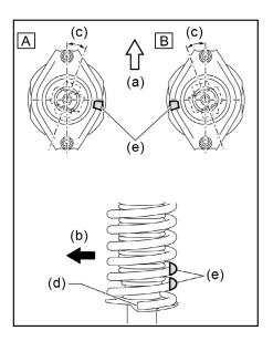
**NOTE:** The end of the coil spring with the gray protective tube (d) must be at installed toward the base of the shock absorber assembly.
