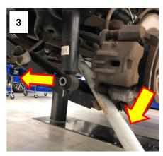
**Step 8)** Remove and discard the other top retaining nut loosened in **Step 5** and remove the affected shock absorber assembly from the vehicle.
