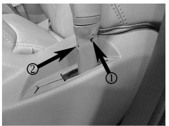
This damage will be in the form of holes (1) or splitting (2).
