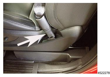
2. Inspect the seat belt tensioner cable cover for damage. Inspect the complete cable cover from the base of the cable to the buckle.
