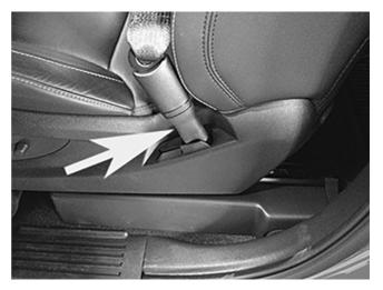
2. Inspect the seat belt tensioner cable cover for damage. Inspect the complete cable cover from the base of the cable to the buckle.
