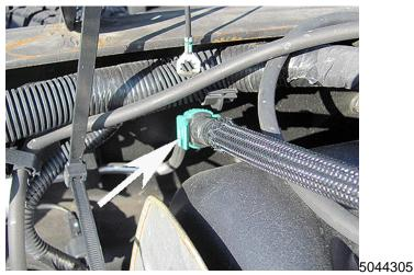
NOTE: The new transfer hose is made of rigid plastic (wrapped in a protective sleeve). **Use extreme care** to not kink the hose when handling and installing.
