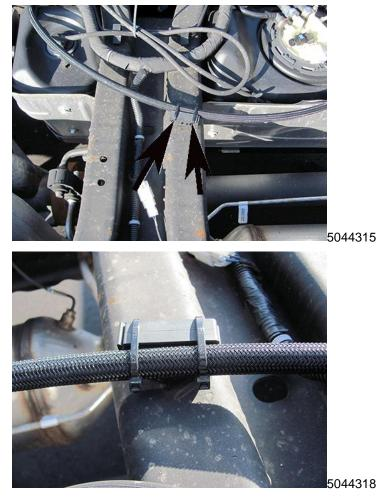
12. Using two wire ties, secure the transfer hose to the frame cross member clip.
