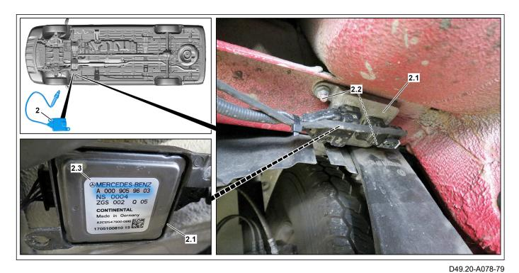
Shown on veh. with engine 642, NO<sub>X</sub>sensor (2.1) control unit upstream of SCR catalytic converter at wheel well crossmember, right side of vehicle
