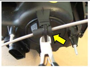
STEP2: exchange position of two adjusting inhibitors, horizontal and vertical beam.
