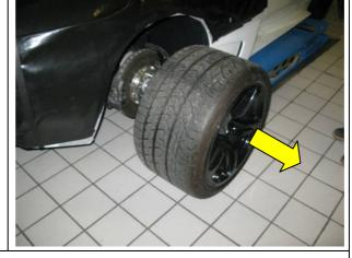
Raise the vehicle higher to make it easier to work under the right wheel arch.
