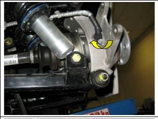
Install the disc brake and tighten the 3 screws.
