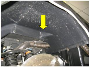
Remove the right rear lateral aerodynamic floor, which is attached by 8 screws
