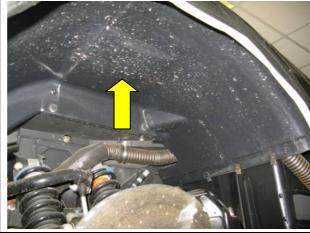
Install the front section of the right rear stone guard and tighten the 10 mounting screws.
