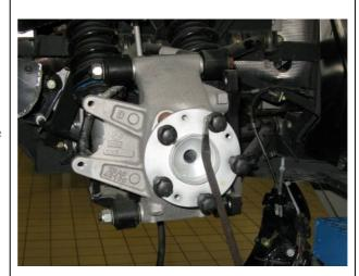
Unscrew the nut and remove the wheel hub mounting pins.
