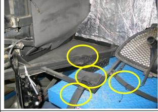
Slide in the new fuel tank as far as it can go so that the grooves on the tank coincide with the retainer straps.
