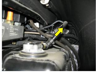
Remove the air intake on the side member after unscrewing the 4 mounting screws, which are located as follows:
