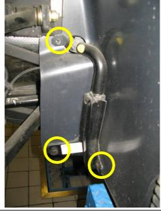
Unscrew the 6 mounting screws and remove the centre section of the right rear stone guard.
