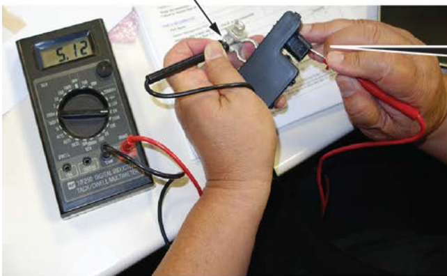
Place the red test lead on Pin 2. Write down the resistance value.
