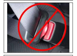
b. Confirm that the driver side seat belt is not latched into the buckle.
