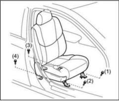
b. Torque the 4 bolts securing the seat to the floorboard in the order shown.
