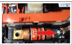
d. Remove the bolt using the insulated 8mm or 10mm magnetic extension and insulated ratchet from the HEV workstation.
