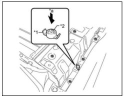
a. Install the battery cover lock striker, then push the button to lock it.
