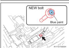
Note: The NEW nut and NEW bolts are marked with blue paint to help identify the replacement parts.
