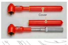
f. Using the insulated magnetic extension and insulated torque wrench from the HEV Workstation, torque the two fuse bolts.
