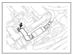
g. Using the insulated magnetic extension and insulated torque wrench from the HEV Workstation, torque the nut for the Buss Bar.
