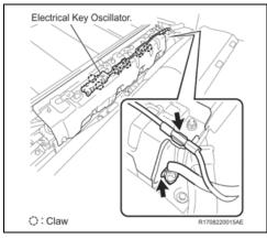
d. Install the 2 claws and 3 clamps of the electrical key oscillator harness.
