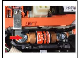
b. Remove the bolt using the insulated 8mm or 10mm magnetic extension (depending on application) and insulated ratchet from the HEV workstation.
