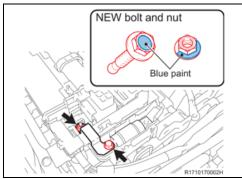
c. Using the insulated magnetic extensions from the HEV Workstation, install the *NEW* nut and *NEW* bolt. Install them hand tight for now.
