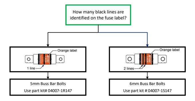
**Note:** If this battery has received service work in the past, it is possible that the fuse currently installed is not the correct size. For example, a 6mm fuse will fit into a 5mm fuse block (using the 5mm bolts). Always select the parts kit to match the thread size of the fuse block.
