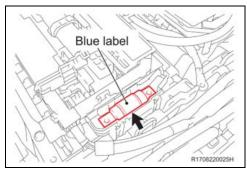
a. Place the *NEW* (blue label) HV fuse into the fuse block, with the part number facing outward. The fuse can be installed in either the left/right or right/left orientation.
