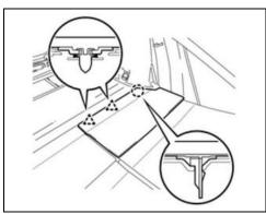
16. INSTALL REAR NO. 2 FLOOR BOARD SUB-ASSEMBLY
