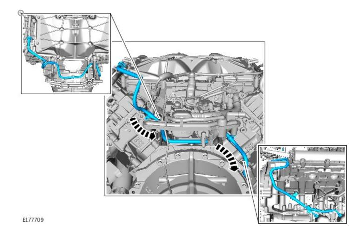
Release the fuel pump supply pipe from the top of the engine.
