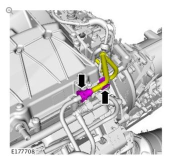
Disconnect the fuel pump supply pipe connector.
