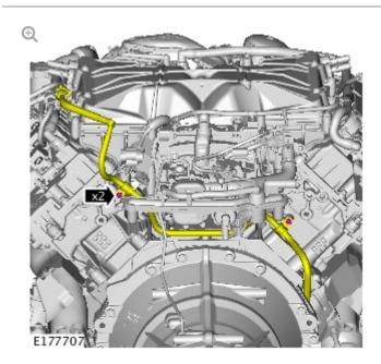
Remove the fuel pump supply pipe bolts.
