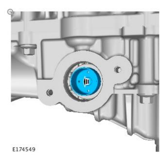
Install the HP fuel pump 2 fuel pump bucket.
