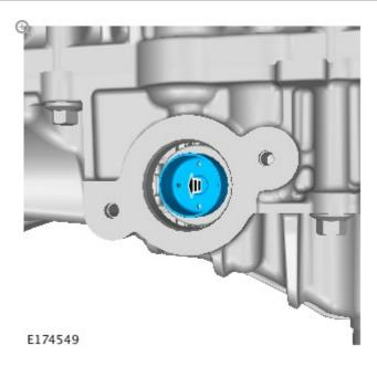
Remove the HP fuel pump 2 fuel pump bucket.
