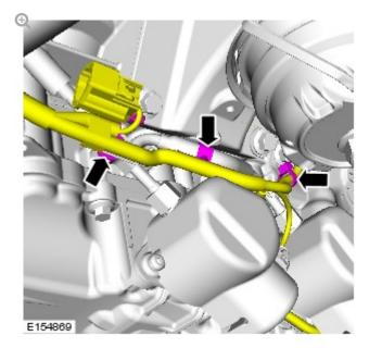
Position the wiring harness to one side.
