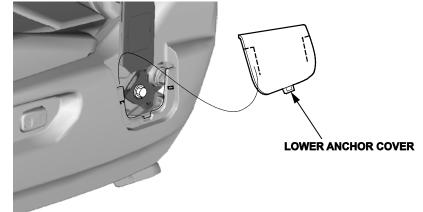
3. Remove the lower anchor bolt.
