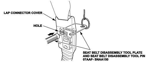
• While pulling the seat belt upward, remove the disassembly tool pin. As soon as you remove the disassembly tool pin from the lap connector, the anchor connector will separate from the lap connector.
