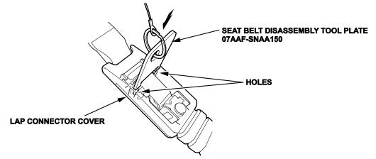
• With the tool inserted, carefully insert the seat belt disassembly tool pin into the hole in the lap connector cover and unlock the lap connector by pushing in on the pin.
