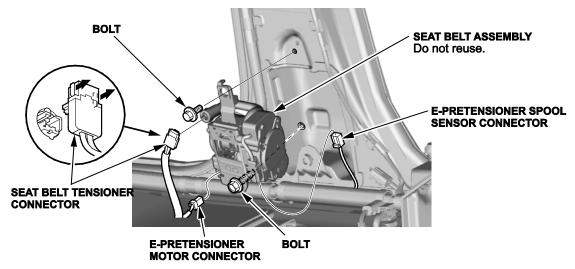
8. If applicable, disconnect the E-pretensioner motor connector and the E-pretensioner spool sensor connector.
