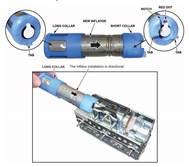
• Slide the inflator in until the plastic collar contacts the bracket. The two tabs should align with the side of the airbag module and the metal tab as shown. There should be no space or gap between the inflator and bracket.
