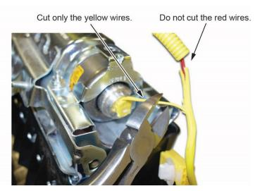
• Strip away about 1 inch of the yellow wire insulation, then twist the wires together.
