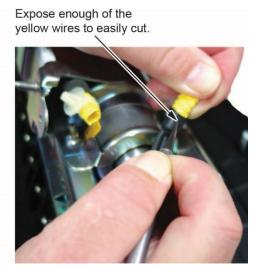
• Strip away about 1 inch of the yellow wire insulation, then twist the wires together.
