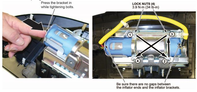
14. Remove the stickers covering the terminals on both sides of the new inflator.
