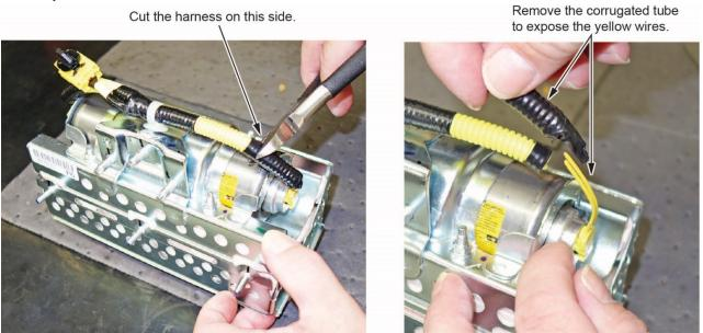
• Strip away about 1 inch of the yellow wire insulation, then twist the wires together.
