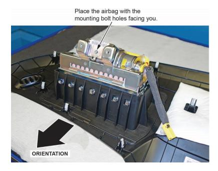
5. Visually inspect the airbag and the inflator for any unusual writing or markings. Refer to IDENTIFYING COUNTERFEIT AIRBAGS.
