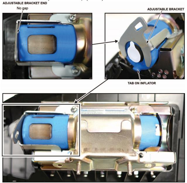
16. Hold the bracket against the inflator, then install the new 5 mm locknuts and torque them in sequence to **4.0 N•m** (34 lb-in).
