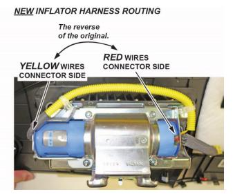
• Connect the red wire connector to the connector on the side with the short plastic cap. Align the "T" shape in the inflator harness connector with the T-shaped inflator connector, then press the connector into place.
