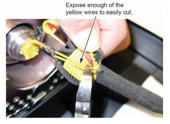
• Strip away about 1 inch of the yellow wire insulation, then twist the wires together.
