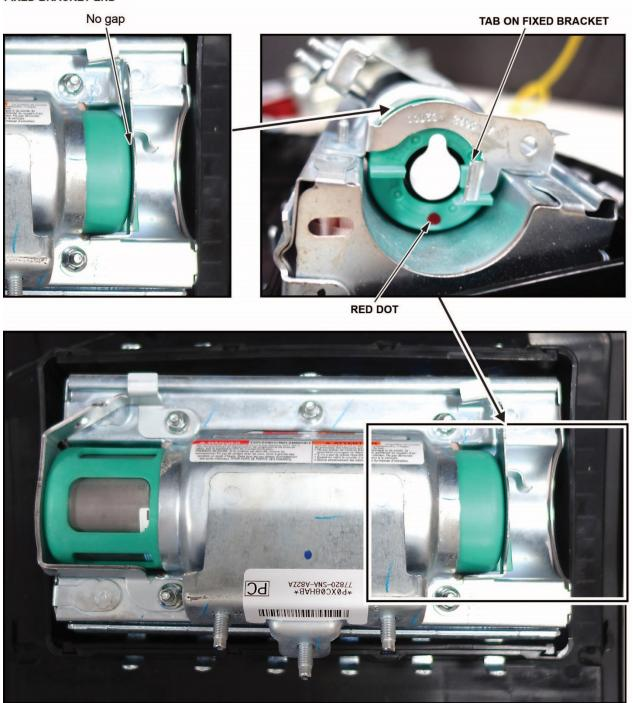
• Install the new bracket included in the kit onto the airbag module. Check there is no space or gap between the inflator and bracket by pushing the bracket against the inflator.
