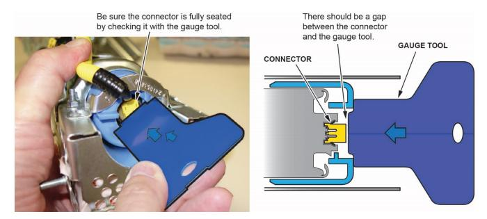
18. Connect the harness to the inflator bracket as shown.
