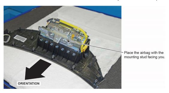
Visually inspect the airbag and the inflator for any unusual writing or markings. Refer to IDENTIFYING COUNTERFEIT AIRBAGS. 6. Peel the label located inside the inflator box from its backing and attach it to the RO. For the warranty claim to be paid, the **replacement inflator part number that you received** must be included in the warranty claim.
