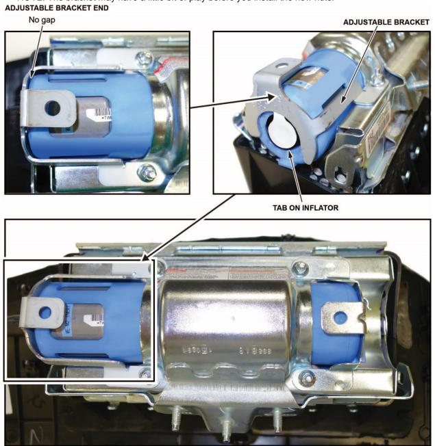
13. Hold the bracket against the inflator, then install the new 5 mm locknuts and torque them in sequence to **4.0 N•m** (34 lb-in).
