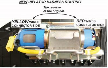
• Connect the red wire connector to the connector on the side with the short plastic cap. Align the "T" shape in the inflator harness connector with the T-shaped inflator connector, then press the connector into place.
