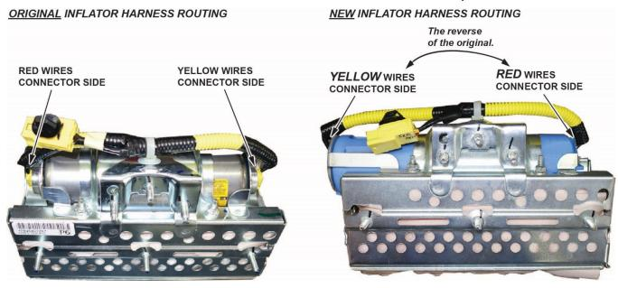
• Connect the red wire connector to the connector on the side with the short plastic cap. Align the "T" shape in the inflator harness connector with the T-shaped inflator connector, then press the connector into place.
