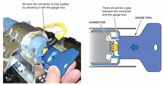
17. Connect the harness to the inflator brackets as shown.
