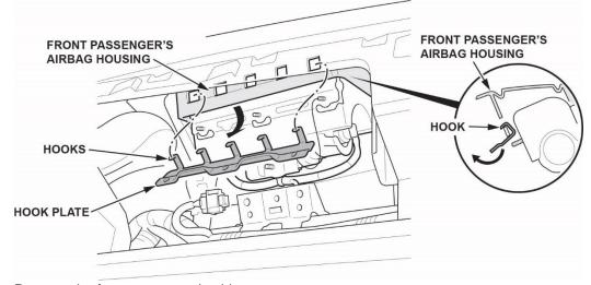
Remove the front passenger's airbag.
