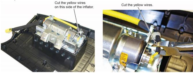
• Strip away about 1 inch of the yellow wire insulation, then twist the wires together.
