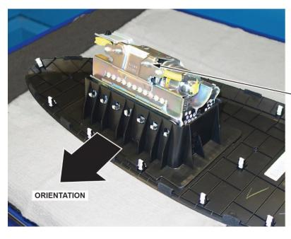
Place the airbag with the mounting studs facing you.
