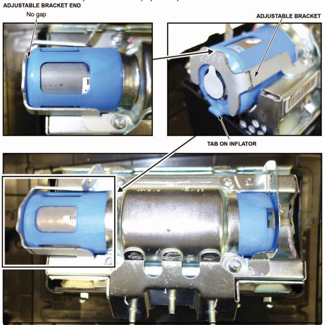
13. Hold the bracket against the inflator, then install the new 5 mm locknuts and torque them in sequence to **4.0 N•m** (34 lb-in).
