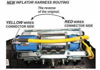
• Connect the red wire connector to the connector on the side with the short plastic cap. Align the "T" shape in the inflator harness connector with the T-shaped inflator connector, then press the connector into place.
