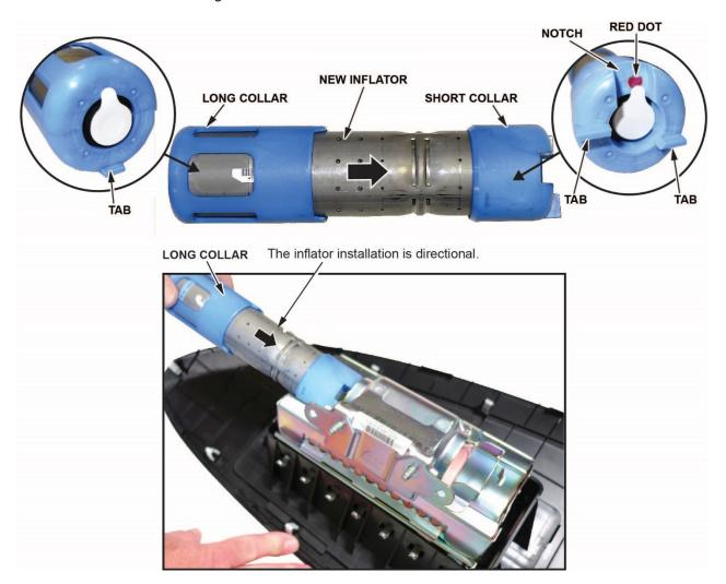
• Slide the inflator in until the plastic collar contacts the bracket. The two tabs should align with the side of the airbag module and the metal tab as shown. There should be no space or gap between the inflator and bracket.
