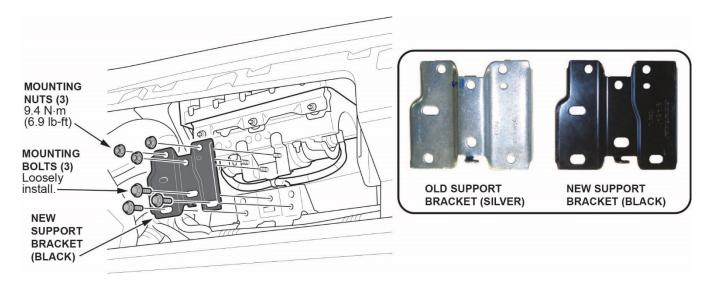
Push the bracket to the left and hold it while torqueing the mounting bolts to 9.4 N-m (6.9 lb-ft).
