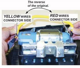
• Connect the red wire connector to the connector on the side with the short plastic cap. Align the "T" shape in the inflator harness connector with the T-shaped inflator connector, then press the connector into place.
