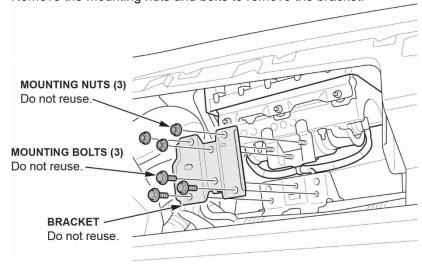
• Remove the mounting nuts from the hook plate.
