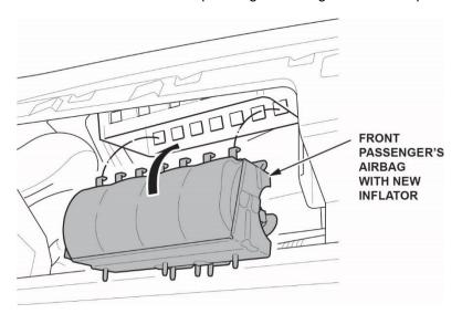
• Insert the hooks of the hook plate into the front passenger's airbag housing.
