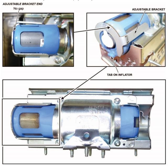
14. Hold the bracket against the inflator, then install the new 5 mm locknuts and torque them in sequence to **4.0 N•m** (34 lb-in).
