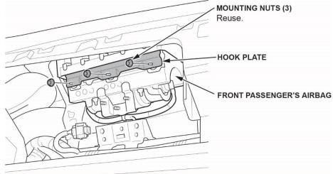
• Release the hooks on the hook plate from the front passenger's airbag housing and remove the hook plate.
