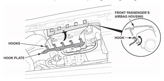
Install the hook plate with the original mounting nuts.
