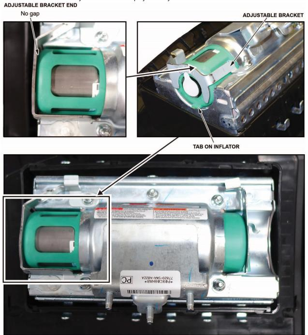
13. Hold the bracket against the inflator, then install the new 5 mm locknuts and torque them in sequence to **4.0 N•m** (34 lb-in).
