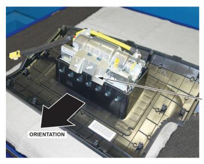
Place the airbag with the mounting stud facing you.
