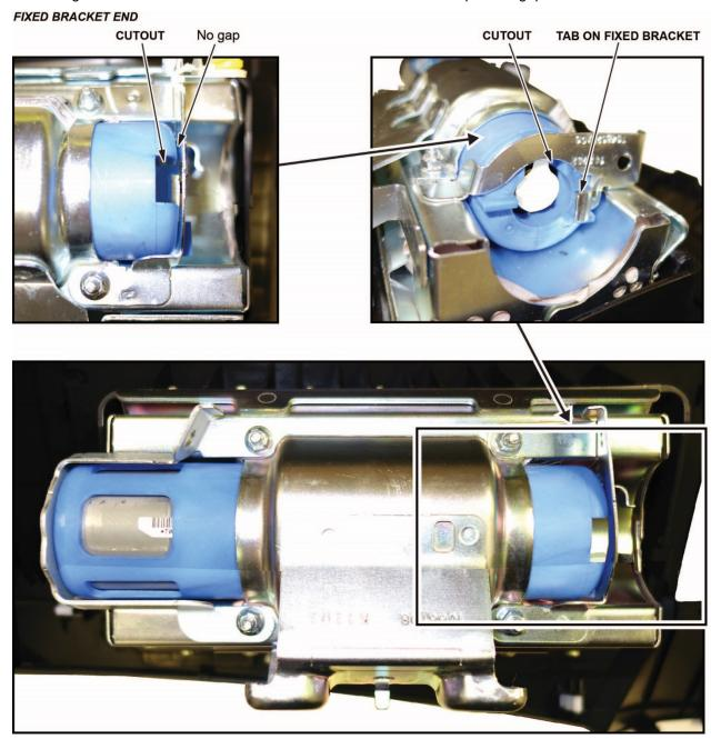
• Install the new bracket included in the kit onto the airbag module. Check there is no space or gap between the inflator and bracket by pushing the bracket against the inflator.
