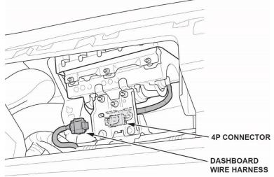
Remove the mounting nuts and bolts to remove the bracket.
