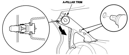
3. Put a shop towel in the opening between the A-pillar and the dashboard to prevent dropping the A-pillar clips.
