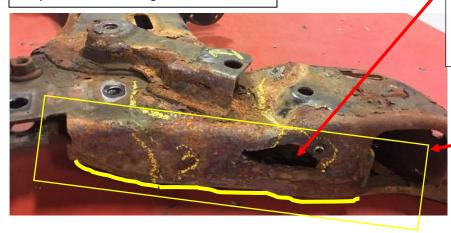
This cross member passes inspection even with the perforation as the bracket supports and covers the hole. If perforation is visible beyond what the bracket covers, the cross member must be replaced as it will fail a state safety inspection for perforation.
