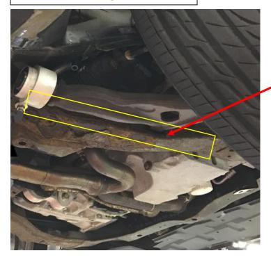
Zone 3 inspection Area: Look for perforation especially along the bottom corner ridge line (this area). If perforation or a crack is present the cross member needs to be replaced.
