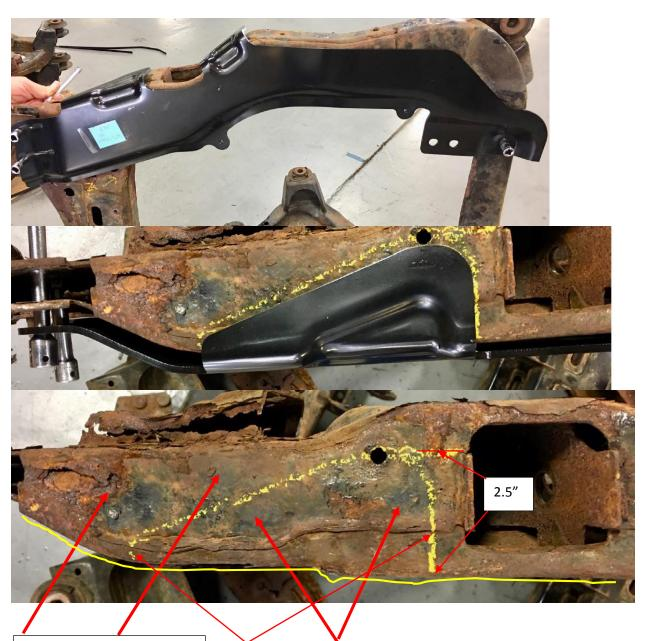
Perforation in this area is not covered by the bracket and will fail State Inspection.
