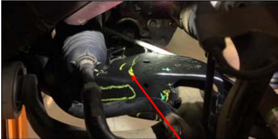
Top Side View: Non-Damaged Cross Member
