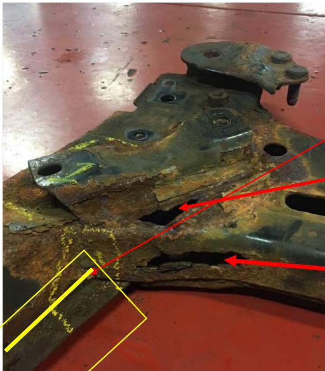
Inside Top View: Damaged Cross member
