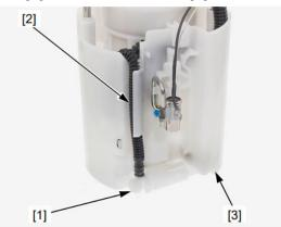
Push the pump flange [1] and remove the Ering [2] from the rod end. Remove the pump flange/rods from the reservoir, then remove the spring [3] from the rod.
