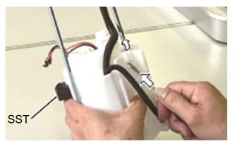
6. Remove the strainer bracket [1] from the strainer case by releasing the tab [2].
