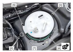
3. Remove the O-ring [4]. Clean the O-ring seating area of the fuel tank, and be sure that no foreign materials enter the tank.
