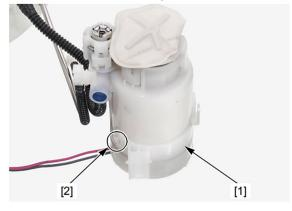
7. Remove the fuel pump/filter assembly [1] from the strainer case [2] by releasing the three tabs [3].
