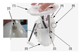
Insert the protruding part of the Special Service Tool (SST) in the lock tab (under the claw). Press the SST up until it clicks. Repeat this process using a second SST for the second lock tab.
