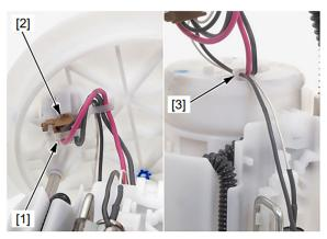
2. Remove cap A [1] and release the return hose [2] from the reservoir [3].
