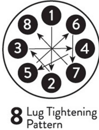
Figure 8 - Lug Tightening sequence
