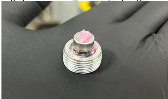
Photograph of the integrated cap, spring, end cap
