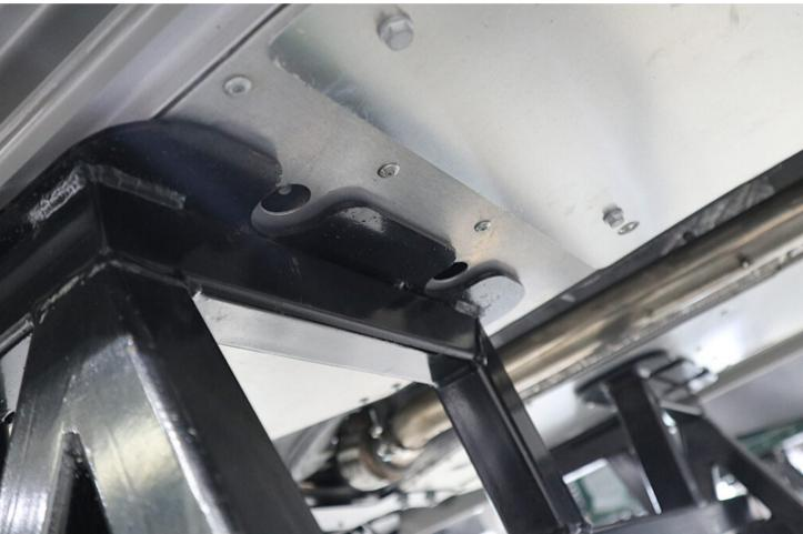
$\cdot$  Underneath the vehicle, fit the (x3) new footwell base plate retaining nuts (as supplied as part of the kit).
