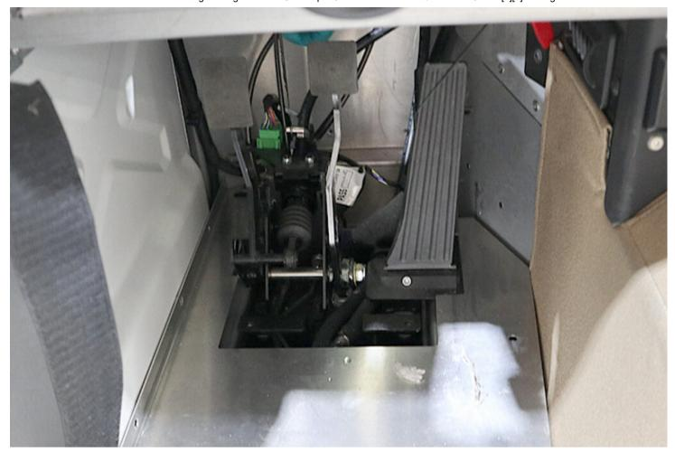
• Refit the electrical connectors on the pedal box which connects it to the main vehicle harness.
