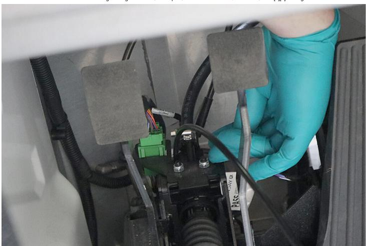
• Refit the clutch pipe into the back of the clutch master cylinder and make sure the retaining clip is secured correctly.
