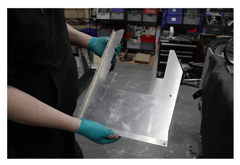
• Refit the footwell base plate. (It may be necessary to adjust the position of the pedal box to access to the base plate).
