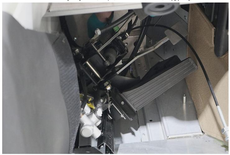
• Fit the new (altered) pedal box into the vehicle.
