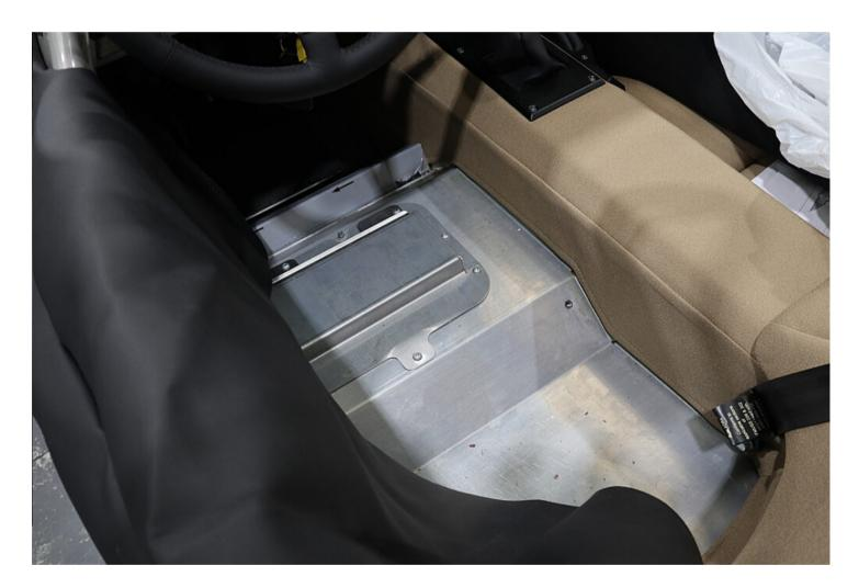
• Remove the front seat base from the driver's side by removing the (x2) bolts with a 4mm hex key.
