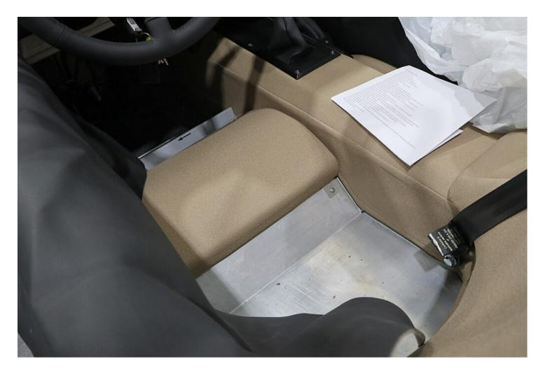
• Remove the rear seat base from the driver's side by lifting it upwards, disconnect the heated seat (if fitted).
