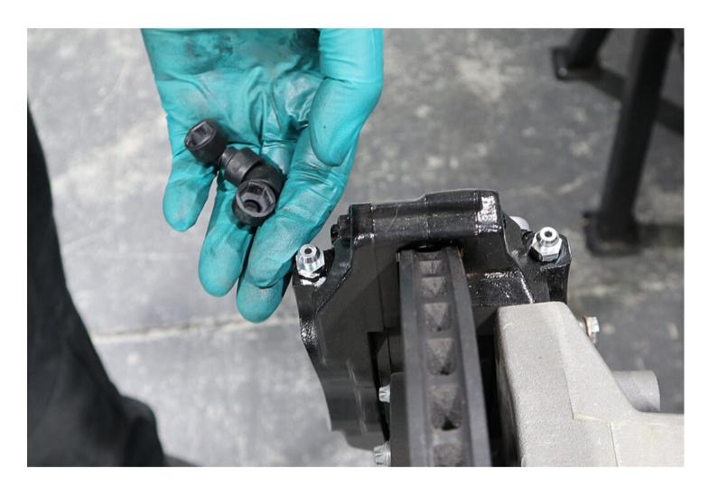
When the first front brake calliper is finished and as much brake fluid is removed as physically possible, carefully remove the vacuum pump unit. Be sure to clean any spillages as the pipe is removed.
