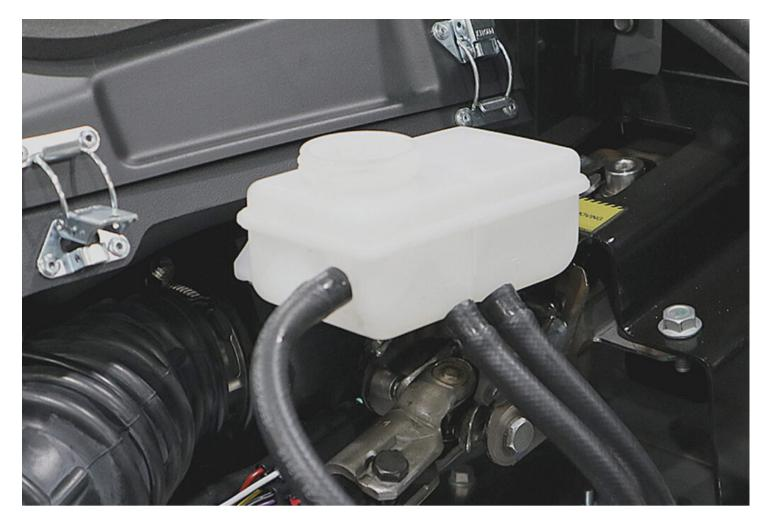
• Undo the hose clamps on the brake fluid reservoir for master cylinder and clutch feed lines using a 7mm socket and ratchet or a flat head screwdriver.
