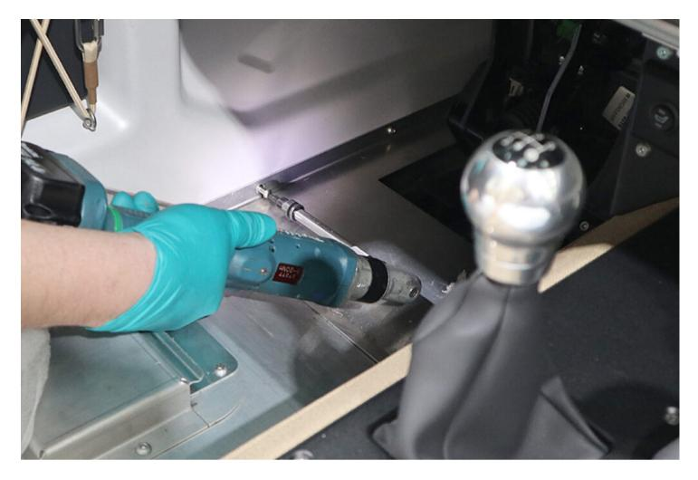
• Remove the accessible bolts retaining the footwell base plate. Removed the plate and store safely.
