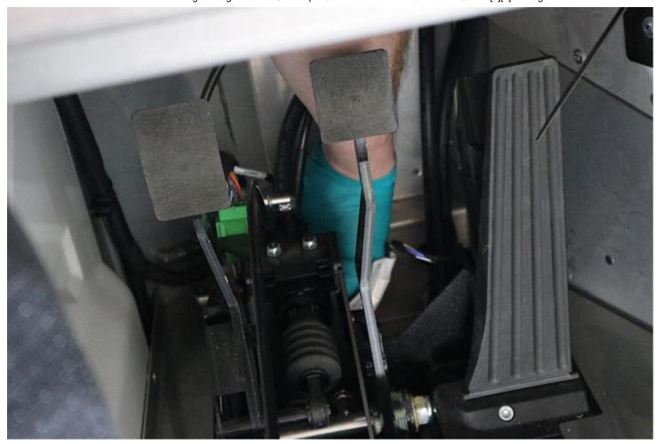
• Disconnect the electrical connectors on the pedal box which connects it to the main vehicle harness.
