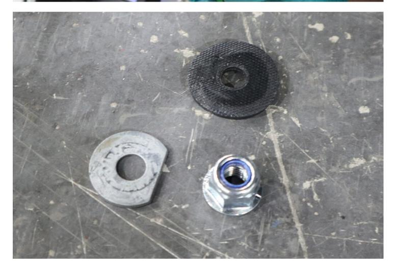
• Underneath the vehicle, remove the inner front footwell base plate retaining nut, washer and rubber washer. Store the washers for re-fitment later – discard the nut, replacements are supplied as part of the kit.
