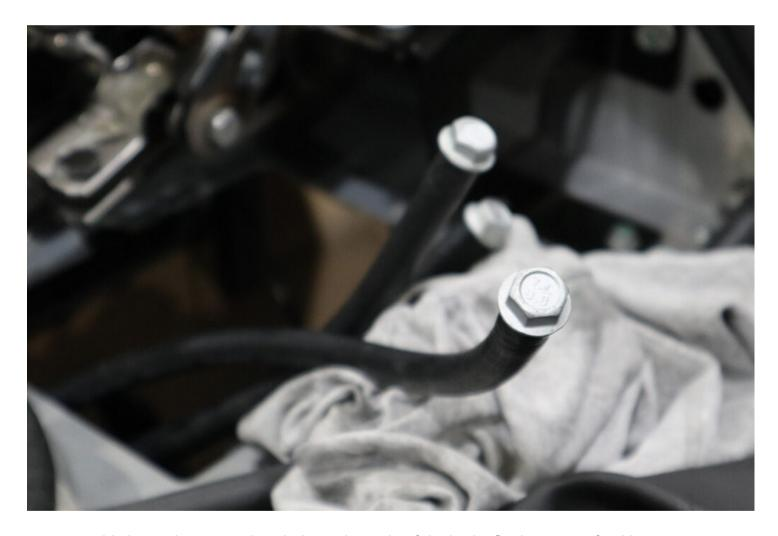
• Use suitable hose clamps or place bolts in the ends of the brake fluid reservoir feed lines to prevent fluid leaks.
