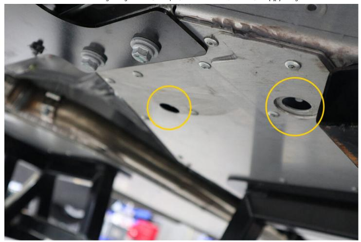
• Underneath the vehicle, remove (x4) grommets underneath the footwell base plate.
