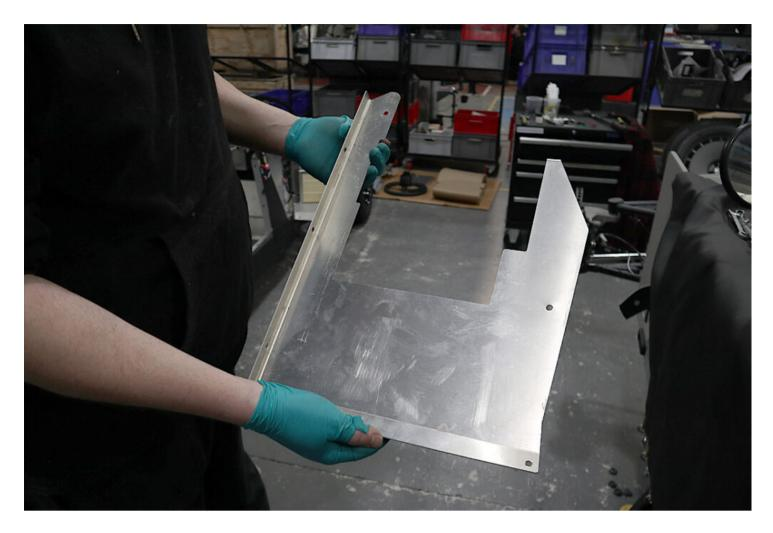
• Remove the footwell base plate. (It may be necessary to adjust the position of the pedal box to access to the base plate).
