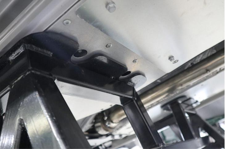
• Underneath the vehicle, remove the remaining (x3) footwell base plate retaining nuts. – discard the nuts, replacements are supplied as part of the kit.
