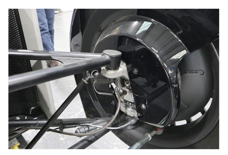
• Undo the (x4) mudguard securing M6 bolts using a 10mm socket and ratchet.
