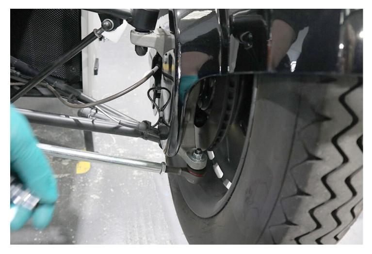
• Unplug the wheel speed sensors on the front left and right wheels.
