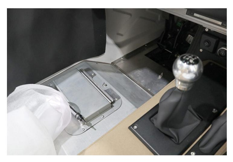
• Remove the foot step retaining bolts using a 4mm socket and ratchet. Remove the foot step from the footwell.
