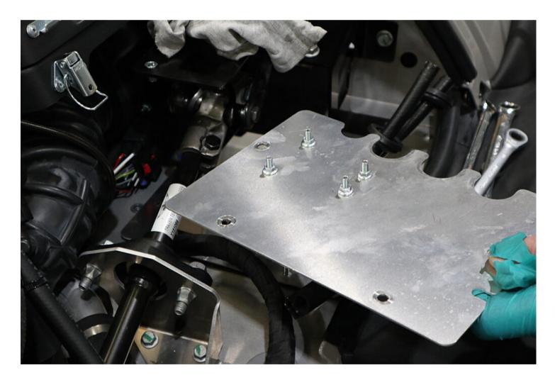
• Reft the pedal box closing plate. Use a 10mm socket and ratchet to refit the bolts.
