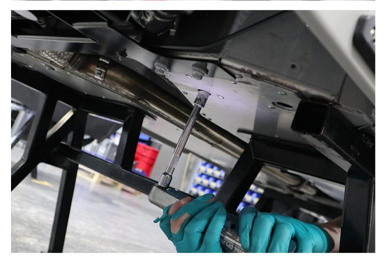
• Refit the inner front footwell base plate retaining washer and rubber washer. Then using the new nuts (as supplied as part of the kit) Torque up to **24Nm** using a 13mm socket and torque wrench.
