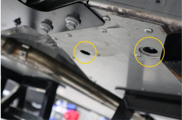
• Underneath the vehicle, refit the (x4) grommets underneath the footwell base plate.
