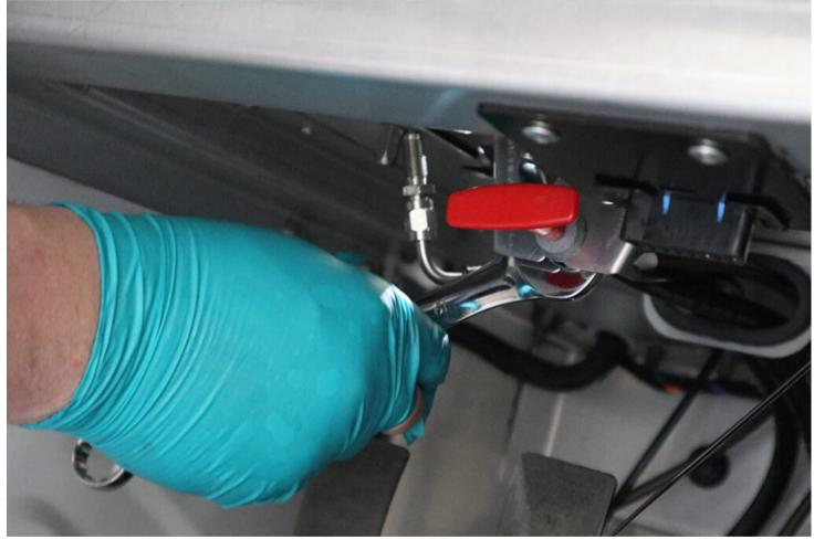
• Use a 19mm spanner to refit the pedal box position adjustment cable.
