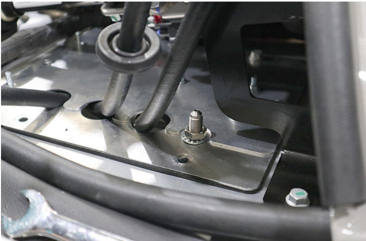
• Use a 15mm socket and ratchet to refit the rear brake union to the bulkhead closing plate.
