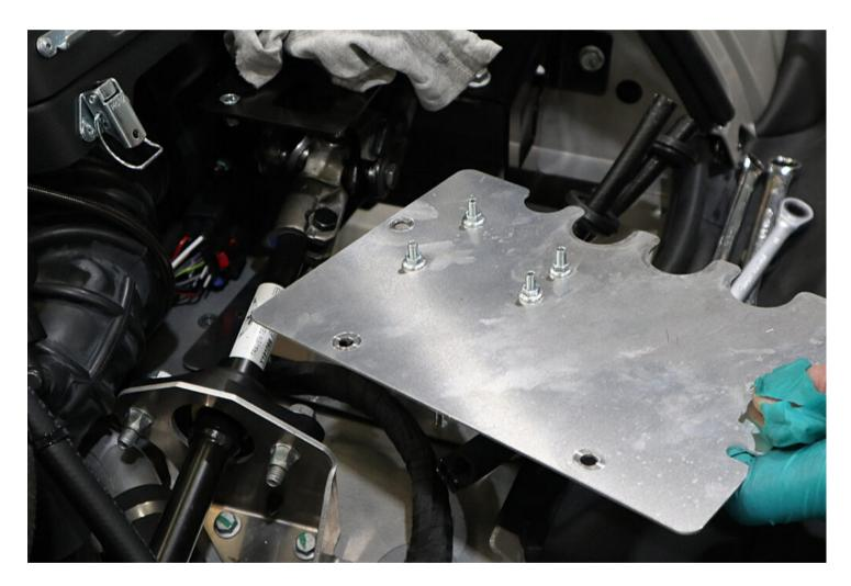
• Use a 10mm socket and ratchet to remove the remaining bolts to fully remove the pedal box closing plate.
