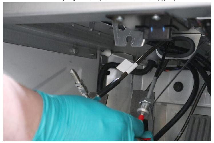
• Use a 19mm spanner to remove the pedal box position adjustment cable.
