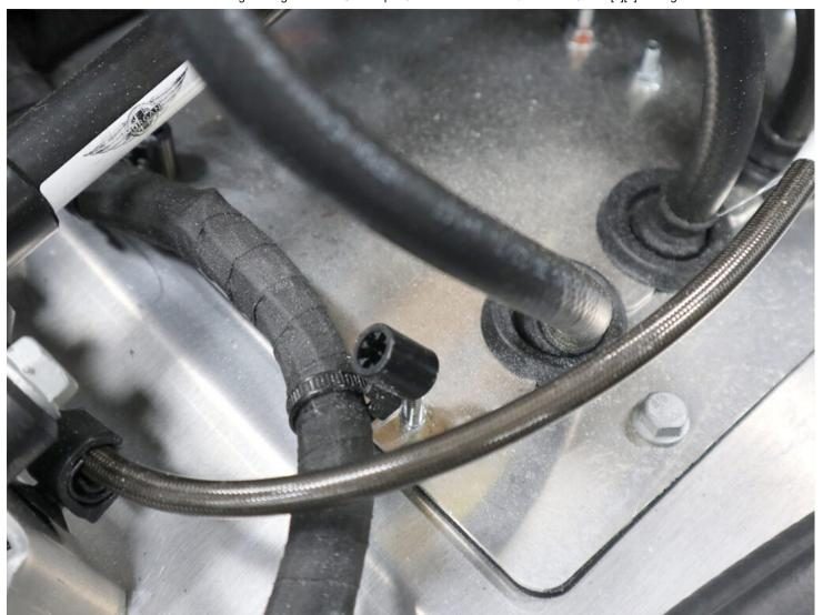
• Using a trim tool (shown opposite) or similar, to very carefully lift up and remove the cable tie push fit clips (x2) to release the wiring harness to the bulkhead closing plate.
