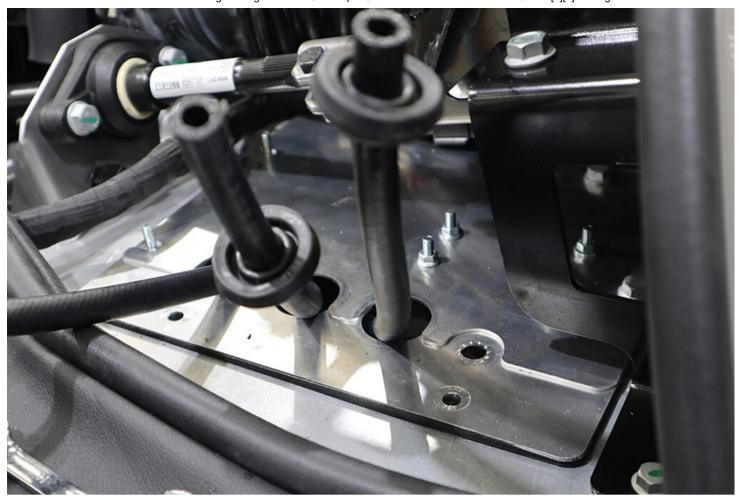
• Use a 15mm socket and ratchet to remove the rear brake circuit union from the bulkhead closing plate.
