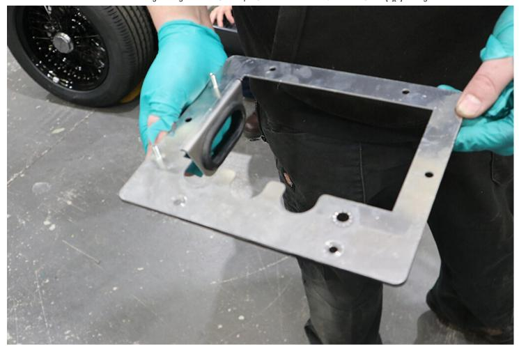
• Thread the brake fluid reservoir feed lines through the closing plate.
