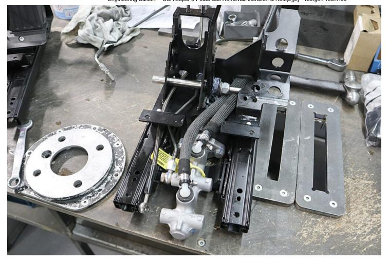
• Feed the rear brake pipe to the new pedal box.
