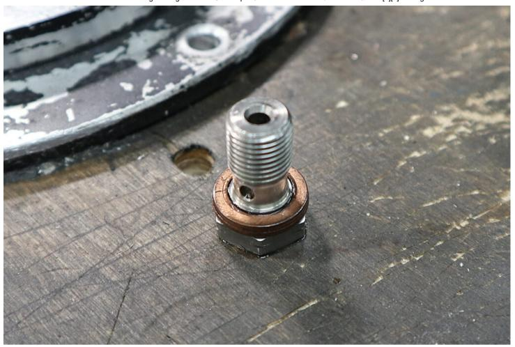
• Use a 14mm spanner to undo the bolt to remove the rear brake pipe from the old brake master cylinder on the old pedal box.
