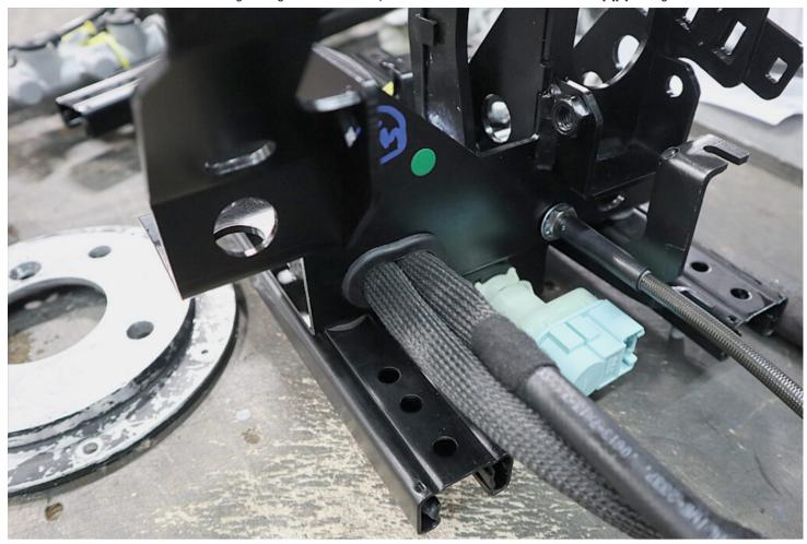
• Fit the grommets to the feed lines and secure using a flat head screwdriver.
