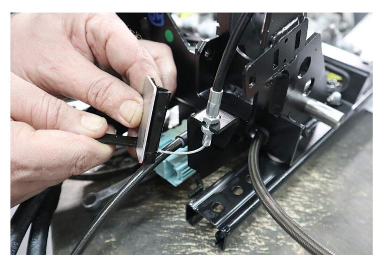
• Fit the adjustment lever retaining plate to the new pedal box.
