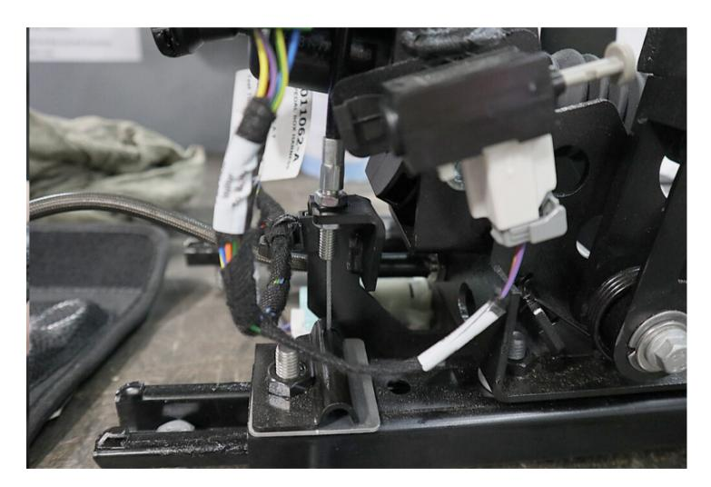
• Remove the adjustment lever from the old pedal box by undoing the nut with a 10mm spanner.
