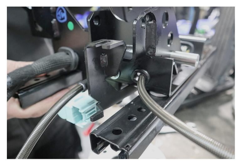
• Fit the grommet for the rear brake pipe to the new pedal box and secure using a flat head screwdriver.
