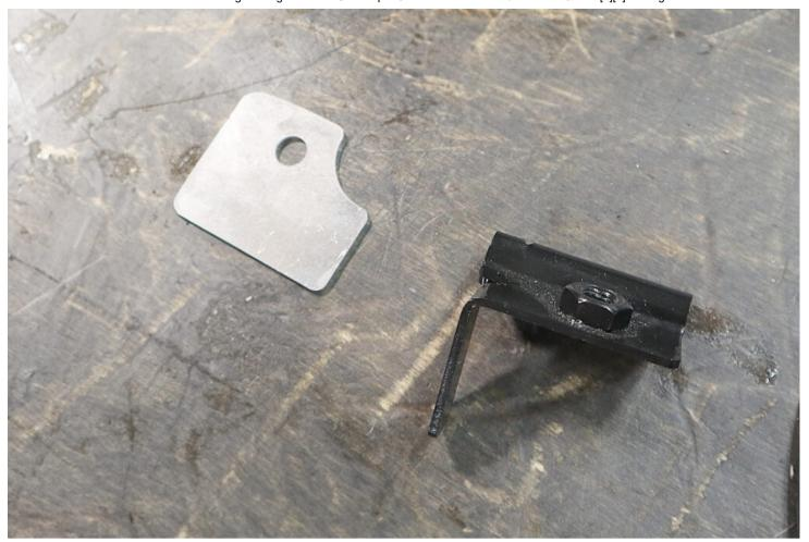
• Remove the adjustment lever retaining plate from the old pedal box.
