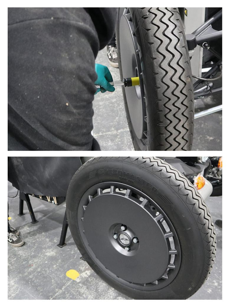
• Refit both front wheels. Refit the (x4) wheel nuts using a 19mm socket and breaker bar or impact gun (if available).
