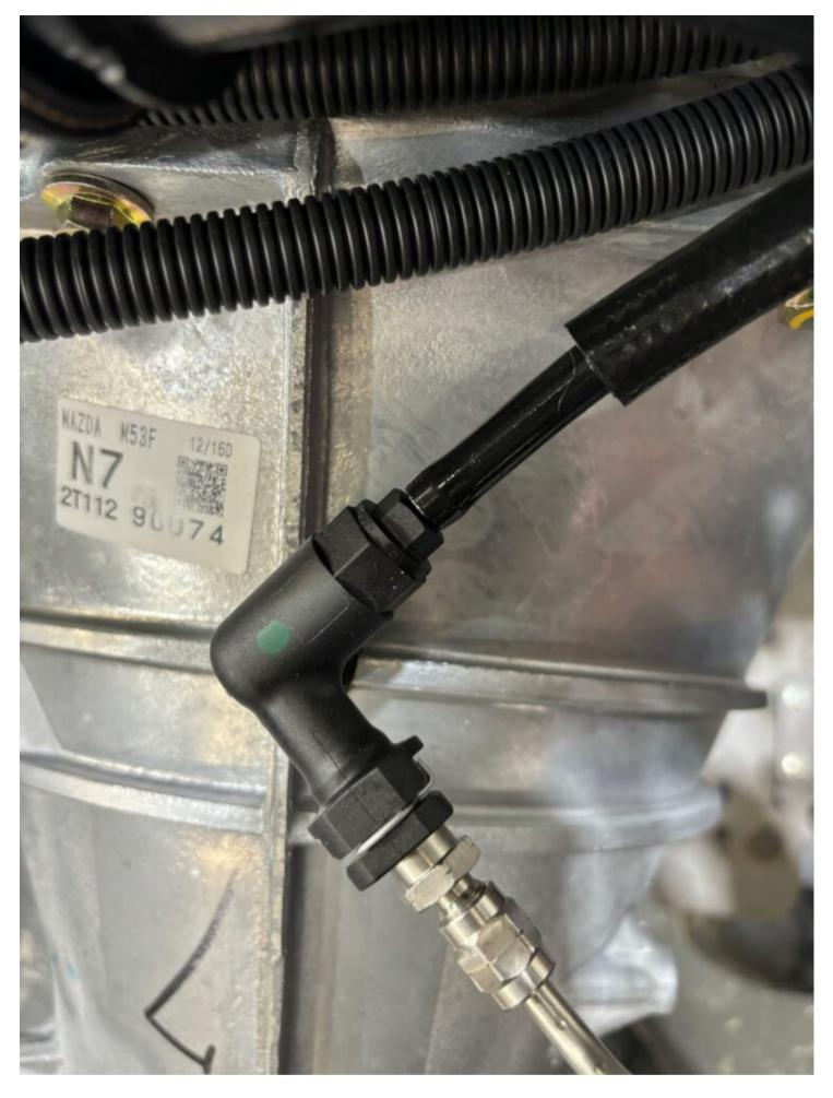
• Attach vacuum filling unit to the clutch master cylinder. Undo the bleed nipple using an 11mm spanner.
