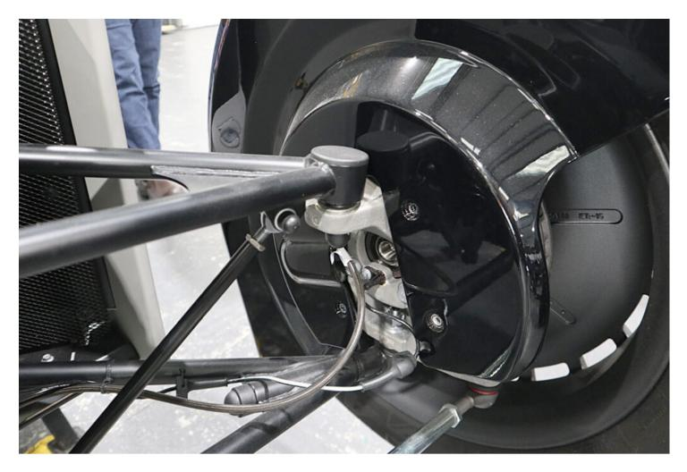
• Refit the (x4) mudguard securing M6 bolts using a 10mm socket and torque wrench. Tighten the bolts to **10Nm**.
