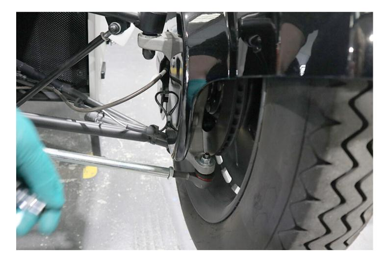
• Plug the wheel speed sensors back in on the front left and right wheels.
