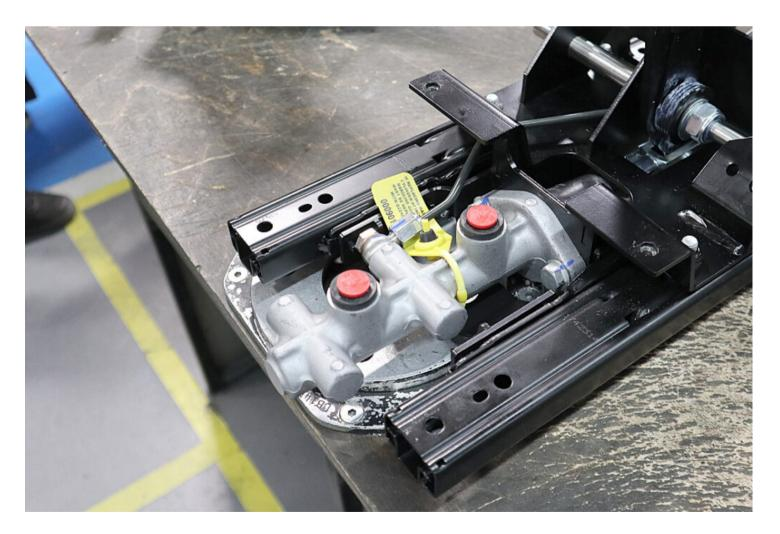
• Remove the bungs from the new supplied pedal box.
