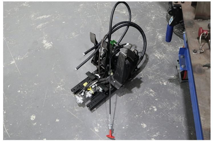
• Remove the pedal box from the vehicle.
