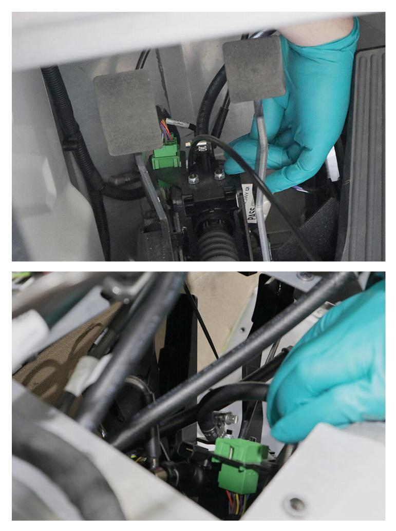
• Release the clip on the back of the clutch master cylinder and remove the clutch pipe.
