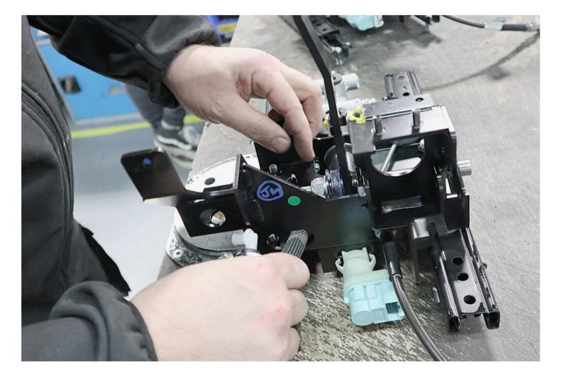
${\boldsymbol{\cdot}}$  Feed the removed lines into the new pedal box.
