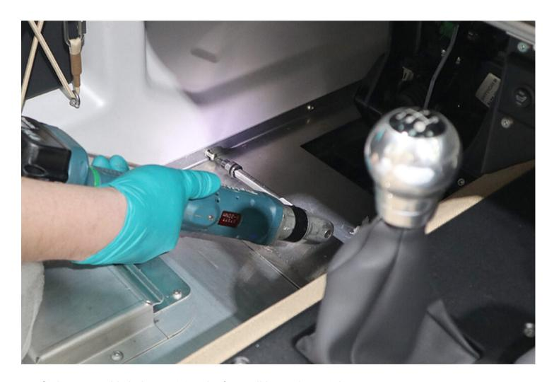
ullet Refit the accessible bolts retaining the footwell base plate. Tighten to  ${f 10Nm}.$
