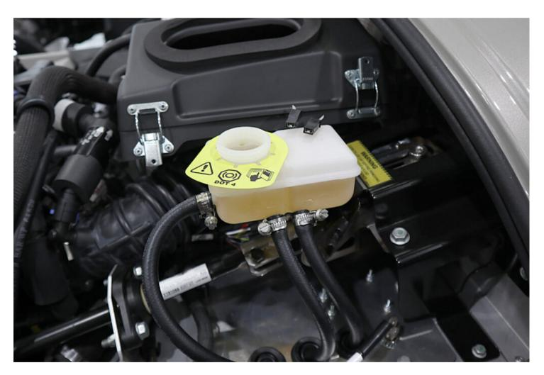
• Refill the brake reservoir with brake fluid.
