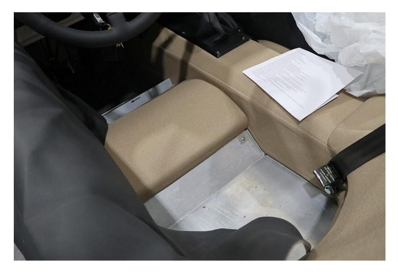
• Refit the heated seat connector (if fitted) and refit the seat base to the vehicle.
