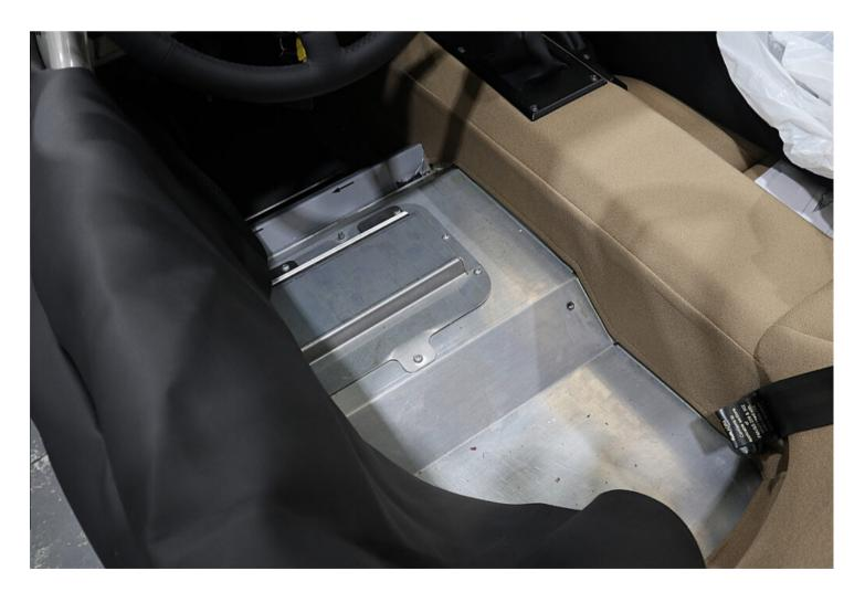
$\cdot$  Refit the front seat base to the driver's side and refit the (x2) bolts with a 4mm hex key.
