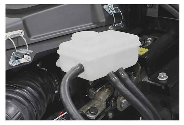
• Refit the clutch master cylinder and brake master cylinder feed pipes to the brake fluid reservoir.
