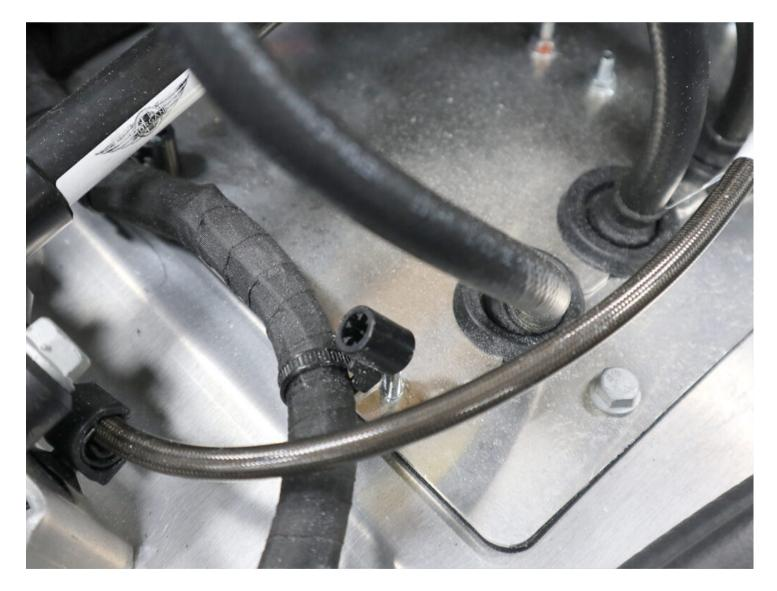
• Refit the cable tie push fit clips (x2) to secure the wiring harness to the bulkhead closing plate.
