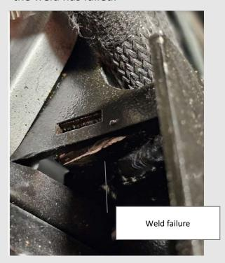
The below photo shows where the connection to the master cylinder has become disconnected due to weld failure of the mounting plate where the master cylinder is fixed. This resulted in the master cylinder being able to move as the pedal is depressed as part of normal braking operation:-
