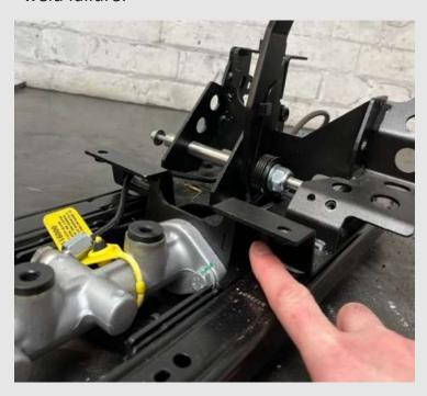
Photo of the defective part where the weld has failed:-
