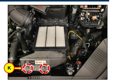
9. Remove the air cleaner assembly (L).
