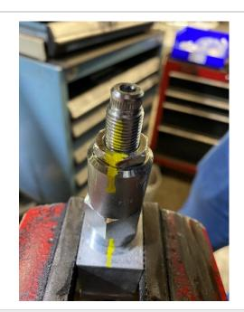
Thread the branch tee in to the port marked 1.
