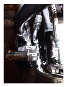
13. Slide any loose hose loops back into the skid and secure away from any moving parts.
