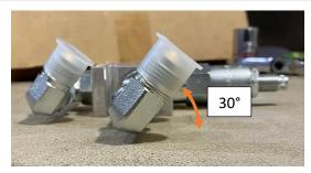
Tighten all fittings, holding each fitting as it is tightened to maintain the angles.
