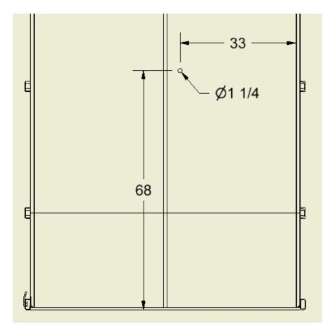
Hole dimensions. The rear of the box is down. The door is not shown.
