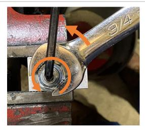
Turn the adjustment screw in 3 full turns. Tighten the jam nut while holding the adjustment screw.
