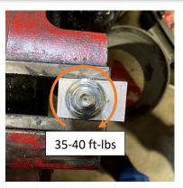
Mark the valve body and cartridge with a line of cross check or a paint pen.
