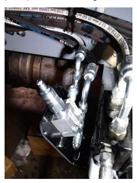
11. Install the dump up hose jumper (2931XZ) from the tee fitting on the side of the valve marked "UP" to the control valve and install on the port that the dump up hose was removed from.
