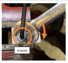
Mark the cartridge threads and body with a line of cross check or a paint pen.
