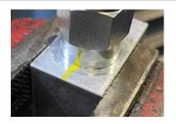
Loosen the adjustment jam nut with a 3/4 in wrench and unscrew the adjustment screw with a 3/16 in hex wrench until it stops.
