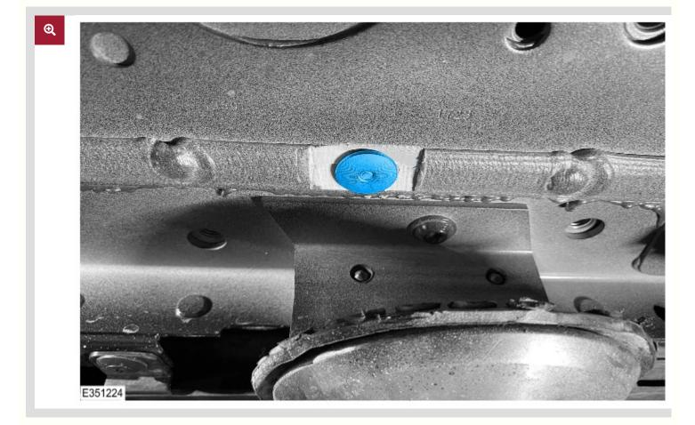
8. Apply a JLR approved sealer over the installed BSF.
