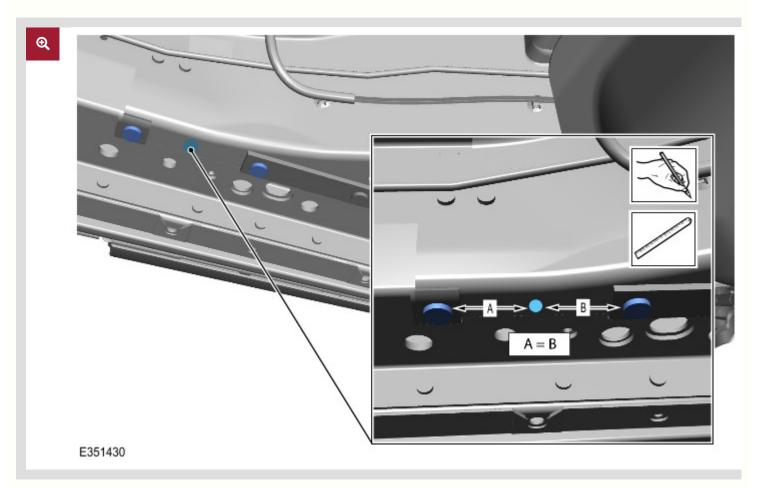
**11.** Using a new or aluminum use only drill bit, drill a 6.5 mm hole in the floor panel.
