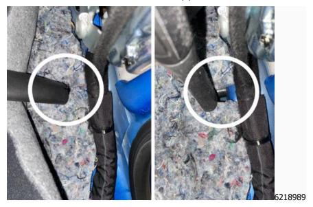
18. Pull the carpet back around the seat belt pretensioner to expose the insulation on the passenger's side of the vehicle.
