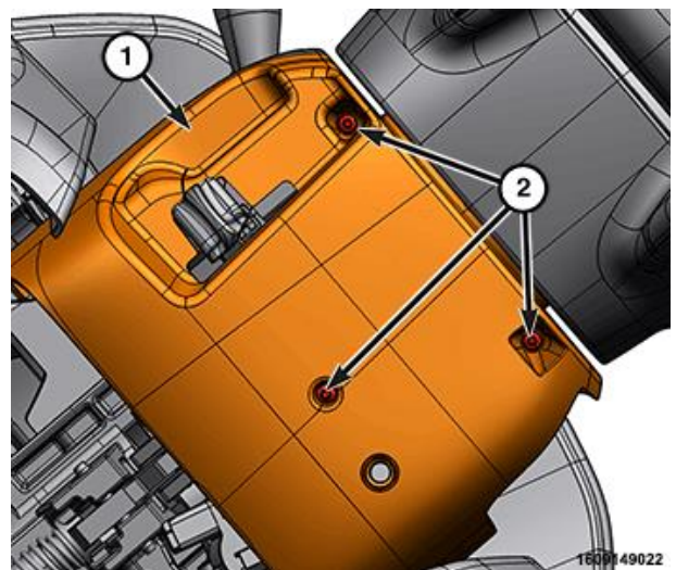
Figure 22 – Steering Column Shroud Screws
