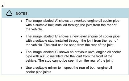
Inspect the fixings/studs on both engine oil cooler pipes.
