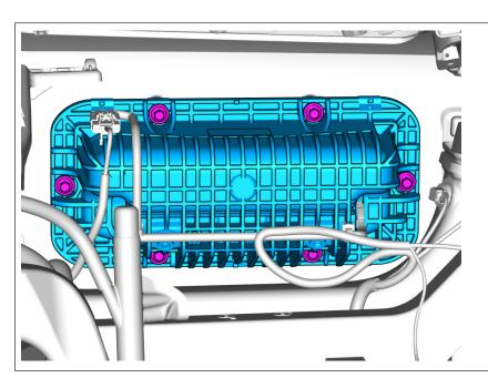
Check that the screws are tightened to the specified torque.
