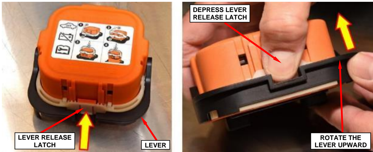
Figure 10 – High-Voltage Manual Service Disconnect First Stage Latch Release (High-Voltage Manual Service Disconnect Removed from Vehicle for Visual Clarity)
