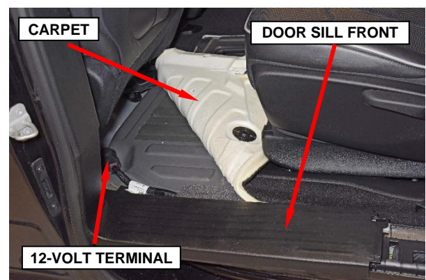
Figure 22 – Door Sill Front and Carpet
