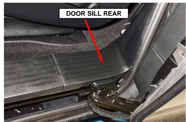
Figure 21 – Door Sill Rear
