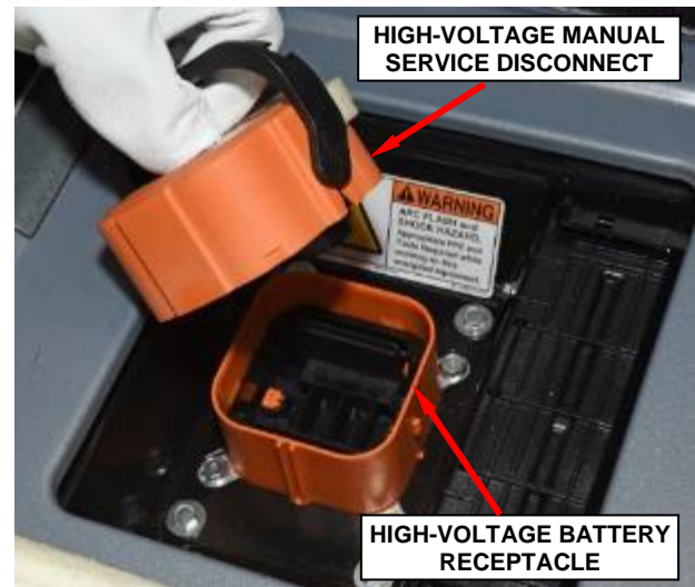
Figure 12 – High-Voltage Manual Service Disconnect and Receptacle
