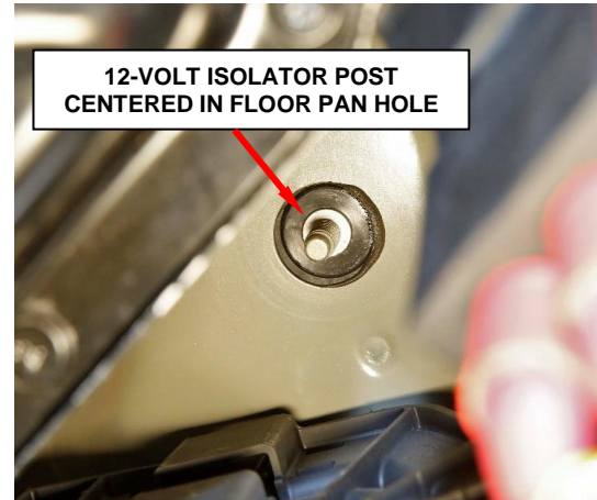
Figure 28 – 12-volt Isolator Post with Attached Guide Removed
