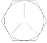
Figure 2. Typical Grade 5 bolt head marking
