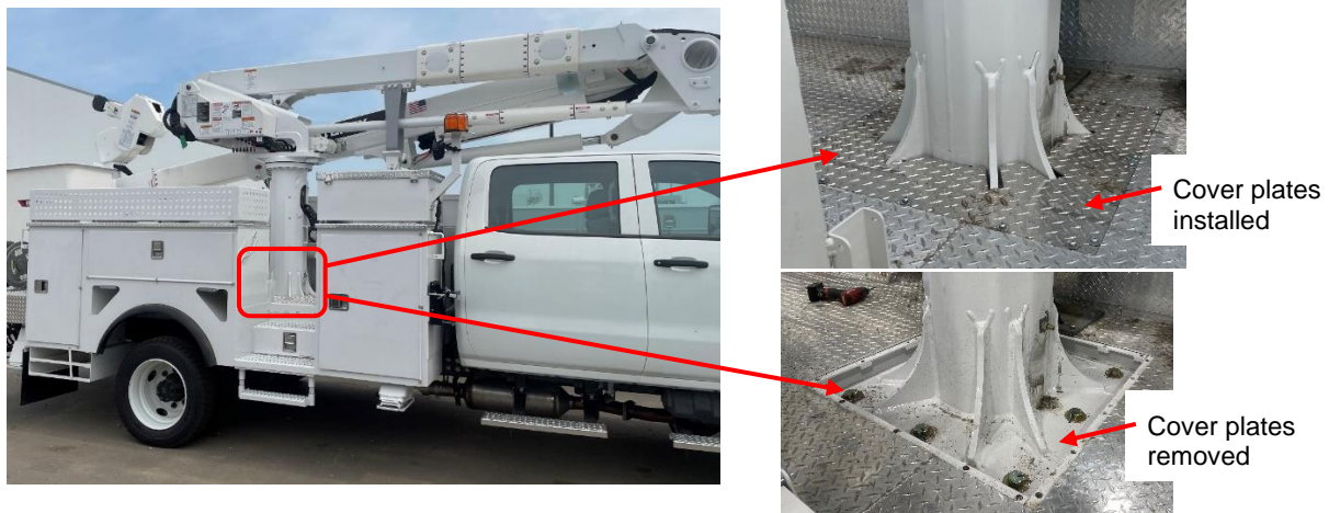
Figure 1. Area of unit to inspect pedestal to sub-base mounting bolts
