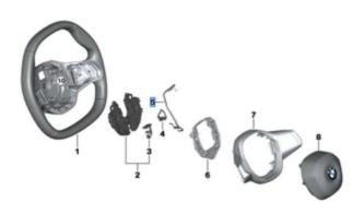
2. Remove the steering wheel airbag following the repair instructions listed in ISTA/AIR 32 34 030 and check the ground screw.
