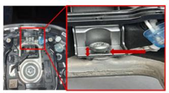
3. Using a magnifying glass, visually inspect the ground screw to determine if the screw is fully seated against the horn plate bracket.
