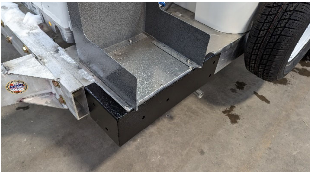
Figure 3a) Streetside Corner Cap top view
